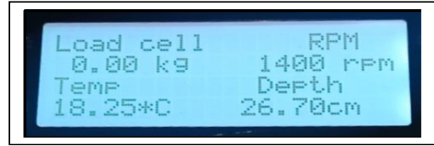
Figure 3: The display on the control board interface of the wear testing machine.
